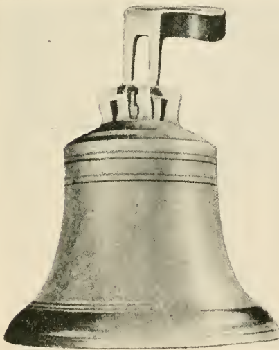
Fig. 35—Method of gating a church bell
